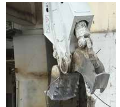
UPX 950 WITH CONCRETE PULVERIZER JAWS
